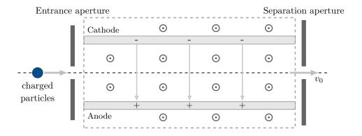
Figure 1: Wien filter's functional principle
